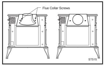
Fig. 16 Reversing the flue collar.
